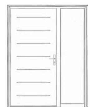
ÉQUATION LARGEUR MAXIMUM AVEC FIXE H 2150 L 1600 FERRAGE UNIQUEMENT SUR DORMANT
